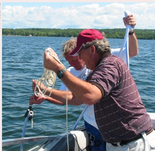
Vermont Lay Monitoring Program volunteer Bob Wood (front) pulls up the weighted end of the hose while partner Chris Demeritt holds the crimp higher than the hose end.
