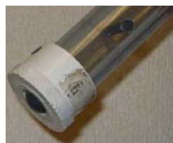
Bottom end of sampler showing the ball in the “closed” position.
