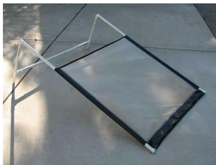
The PVC frame is adjustable to two different heights for use in deep and shallow water.
