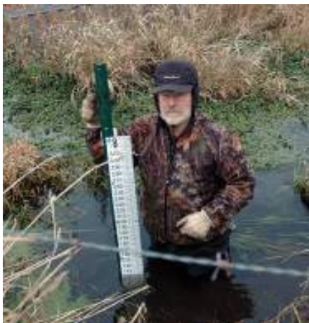
Steve Rankin installs one of the stage/crest gages he designed and built.
