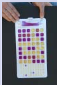
IDEXX Colisure. Wells with a red or magenta color plus fluorescence are positive for E. coli .
