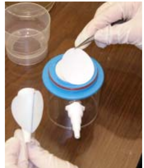
After filtration, the membrane filter is removed and placed on an appropriate medium for the indicator organism.
