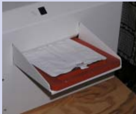
A special sealer must be used to seal off the individual wells in the IDEXX Quanti-Tray.
