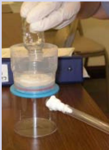
The water sample is filtered, then the filter is placed on Coliscan medium.
