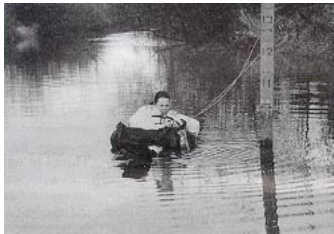
A CRUE student in an inner tube retrieves a Hydrolap (a submersible automated sampler) from the Columbia Slough.
