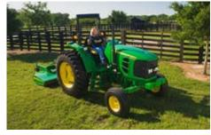
Mow pastures, brush, and roadsides. Rotary cutters, powered by the tractor's PTO, handle tough cutting and mowing jobs, and are perfect for pastures or other big, open spaces. Most rotary cutters are available in several sizes and duty levels.
