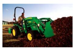
Move dirt piles, silage, gravel, snow, hay bales, or other materials. A front-end loader, one of the most popular attachments for utility tractors, can help you handle just about any material moving chore.
