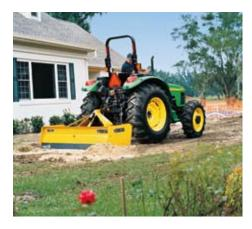
**Dirt or materials work.** If it needs to be smooth as glass, go over it with a box blade, land plane, or other leveling implement to re-grade or fill potholes.
