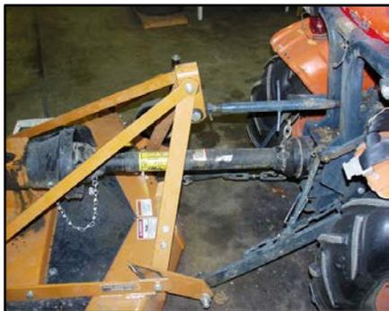
Figure 2. Driveline connected to the tractor
