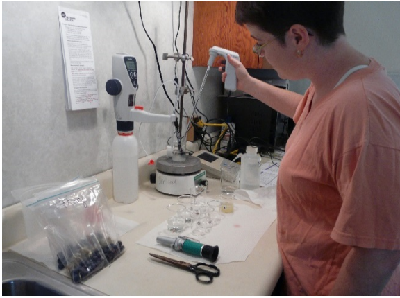
Figure 1: A simple and effective juice field lab can be set up on a bench in the shop, or even on a truck tailgate. Pictured here are (counter clockwise, beginning at lower left): bagged grapes for squeezing; a refractometer for measuring sugars; a pH meter; and a titrator for dispensing NaOH.
