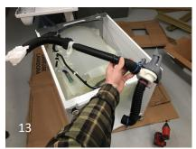
19. Cut the last zip tie but leave the connector on the bottom of the machine.
