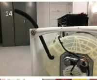
20. Split the cable wrap and extract the wires.
