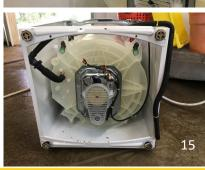
21. Remove the connector and wires from the synchronous motor. These wires are not needed.
