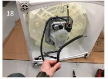
13. Remove the pump and drain tubing by removing (6) 5/16" screws.
