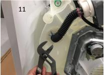
17. Remove the Clear tubing along with the wiring harness. There are some wires inside this harness that will be used.
