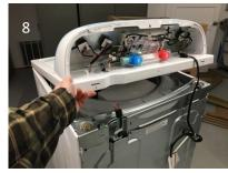
Use a screwdriver to remove the plastic splash guard around the top of the drum. (There are 8 points of attachment, after unhitching ~½ you can just pull up on the ring).
