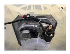
13. Secure both cord connectors to secure the cables coming in and out of the box.
