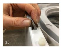
10. Pull the tab to remove the wiring harness from the chassis.
