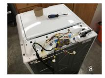
Lift off the top portion of the washer. The front edge snaps into place. Pry to pop it loose.
