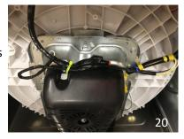
21. Use zip ties to secure the wire to the chassis through the corner bracket as a strain relief.
