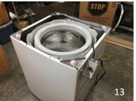
9. Turn the machine upright and mount the electrical box to the side of the appliance using a 2.5" corner bracket. Install it on an angle for ease of use with 1/4" self-tapping screws.
