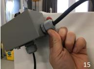
11. Install the cord fittings to the waterproof box and insert the cord from the motor wires, and the appliance power cord into the box, do not pinch the wire down in the connector just yet.
