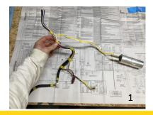
2. Take the wires removed from the cable wrap and separate the white, yellow, green/yellow, and brown from the rest.
