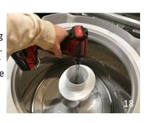
13. Remove the (2) screws securing the top of the machine.
