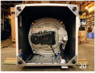
21. Using a 3/8 socket remove the screws (3) from the plastic cover covering the motor and drive belt.
