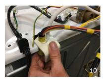
Remove the plastic splash guard around the top of the drum by lifting on the tabs.
