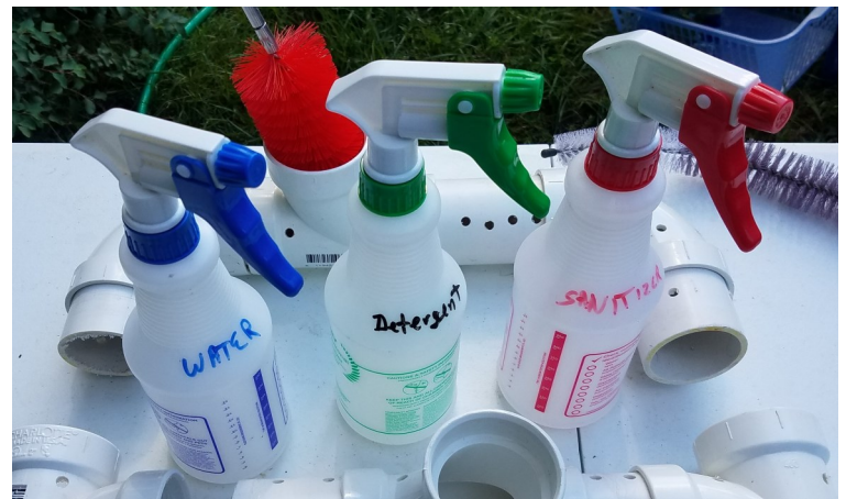
Spray bottles can help ensure coverage in hard to reach spaces on PVC piping. Consider using color-coded bottles for water, detergent, and sanitizer to avoid confusion.
