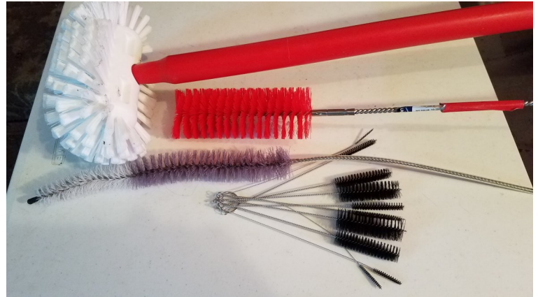
An assortment of brushes including a long handled scrub or tank brush, large diameter bottle brush or flex handle bottle brush, and small diameter (1/2") bottle brush will help to clean hard to reach spaces.
