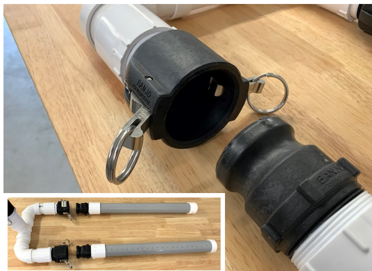
Camlock fittings provide an easy disassembly and reassembly option and make cleaning easier and more effective.
