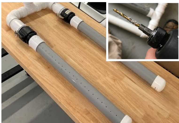
Medium diameter, 1/8" holes spaced at 1 hole per inch seems to be a reasonable compromise for most applications.
