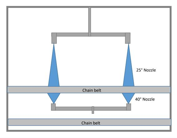
Stage 2 pressure is equal in both spinner arms but the nozzles differ to provide even coverage
