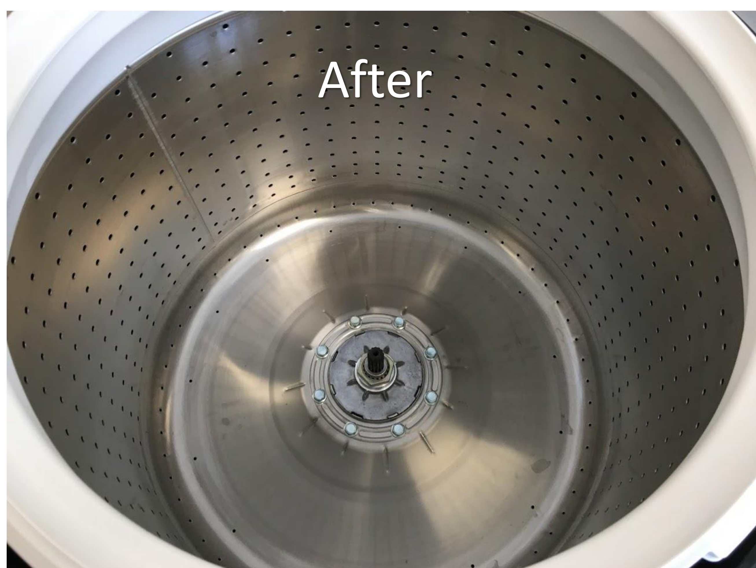
A Speed Queen washing machine like this one costs more up-front. But, it has a smooth, stainless steel drum with an easily removed agitator plate. This makes it easier to clean when used as a greens spinner. A basket insert is used to contain the greens which provides a removable, cleanable food contact surface. This model also does not require additional material to be added to hold a basket insert securely.
