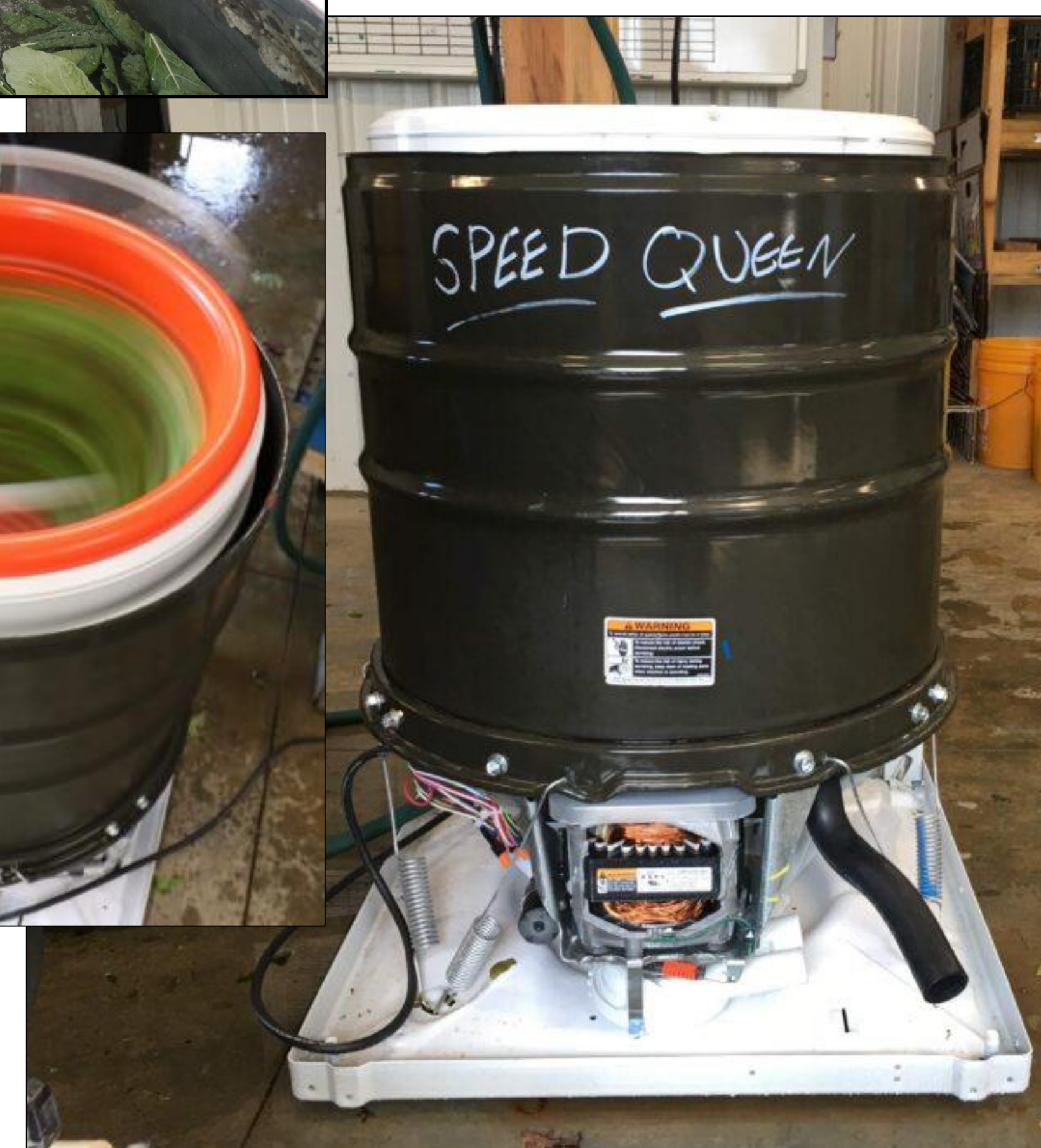
Using basket inserts and removing paneling improved the cleanability of this washing machine greens spinner.
