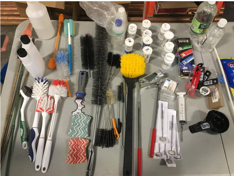
▲ A variety of cleaning tools may be needed to easily reach and completely clean produce wash equipment. From left to right: extension sticks with scrubbers on the end, stiff short brush, toilet brushes, large bottle brush, paint scraper, scrub pads, assorted bottle brushes large to small, long scrub brush, inspection mirror, small bottle brushes, assorted test strips.
