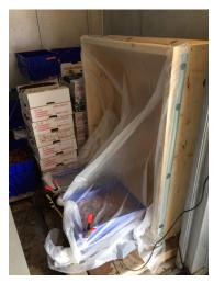
A precooling experiment was conducted to test the performance of a small scale (countertop sized) forced air cooler (FAC) in parallel with product cooled by room cooling. Freshly harvested blueberries (28 lbs) were placed in a walk-in cooler set at 40 °F. In the case of room cooling the product temperature is reduced as a result of simply being in the room with cool air circulating around it. The same mass of product was placed in a small
