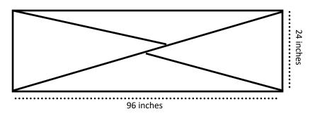
**Side view:** the frame is made from square 1.75 inch steel greenhouse endwall framing material. Foam board is attached on the outside of the framing using Tek Screws. The door is a piece of foam board the size of the front mounted on a channel that allows it to slide. It is held in place by a 2x2 piece of lumber across the front (see picture next to profile)
