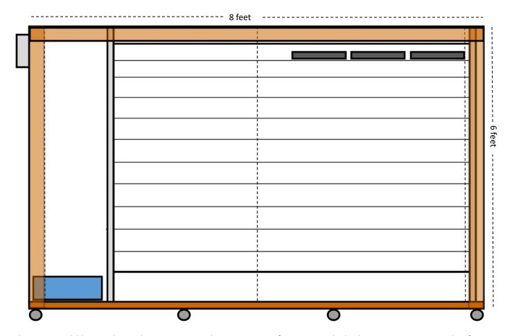
This unit could be easily made to accommodate a variety of spaces, with the box consisting entirely of common lumber. The key technology features of this chamber are the temperature and humidity monitors, which allow the farmer to constantly monitor the chamber despite not living at the farm. Each chamber needs its own monitor, but the cellular relay which conveys information is shared by the two units.
