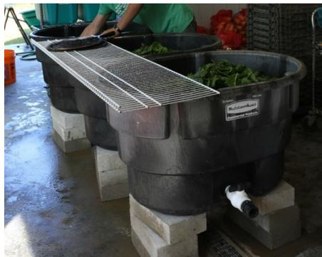
◀ Stock tanks, on cinder blocks for prototyping to find the best working height. Note the use of coated, wire closet shelving above the tanks for holding and draining baskets.
