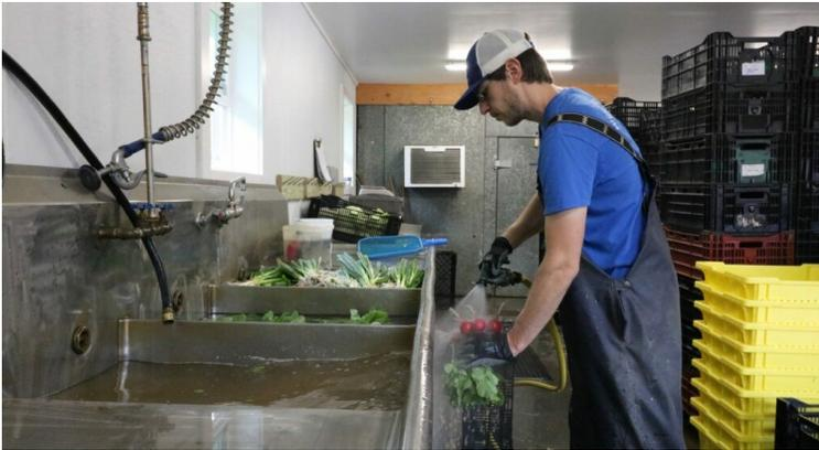
Stainless steel restaurant sinks are desirable because they are large, durable, easy to clean, and fairly easy to find. The restaurant industry transitioned to full stainless construction, so now there are used tables and sinks with stainless tops on galvanized legs available. Full stainless steel equipment is not required for produce washing. The key requirement is that food contact surfaces are smooth and cleanable as appropriate.
