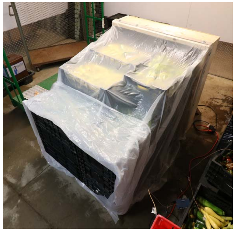
▲ This is a 4 foot tall version of a simple, portable forced air cooler. It is being used to cool a mixed pallet of fresh picked zucchini, summer squash, and peppers.
