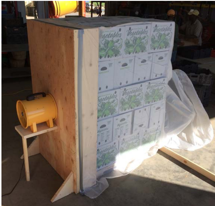
▲ The blower is just placed up to the cut-out hole, on a shelf. This unit has a very simple shelf and feet to add some stability.
