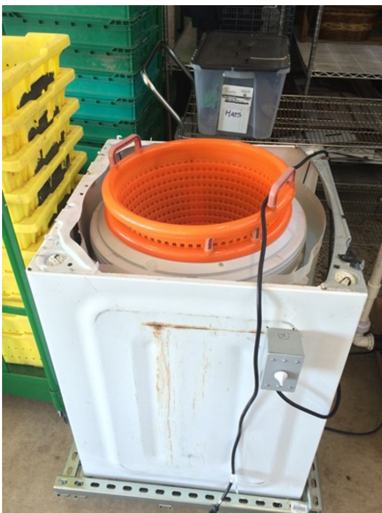
▲ A washing machine conversion using a plastic “fish basket” as an insert and external power switch.
