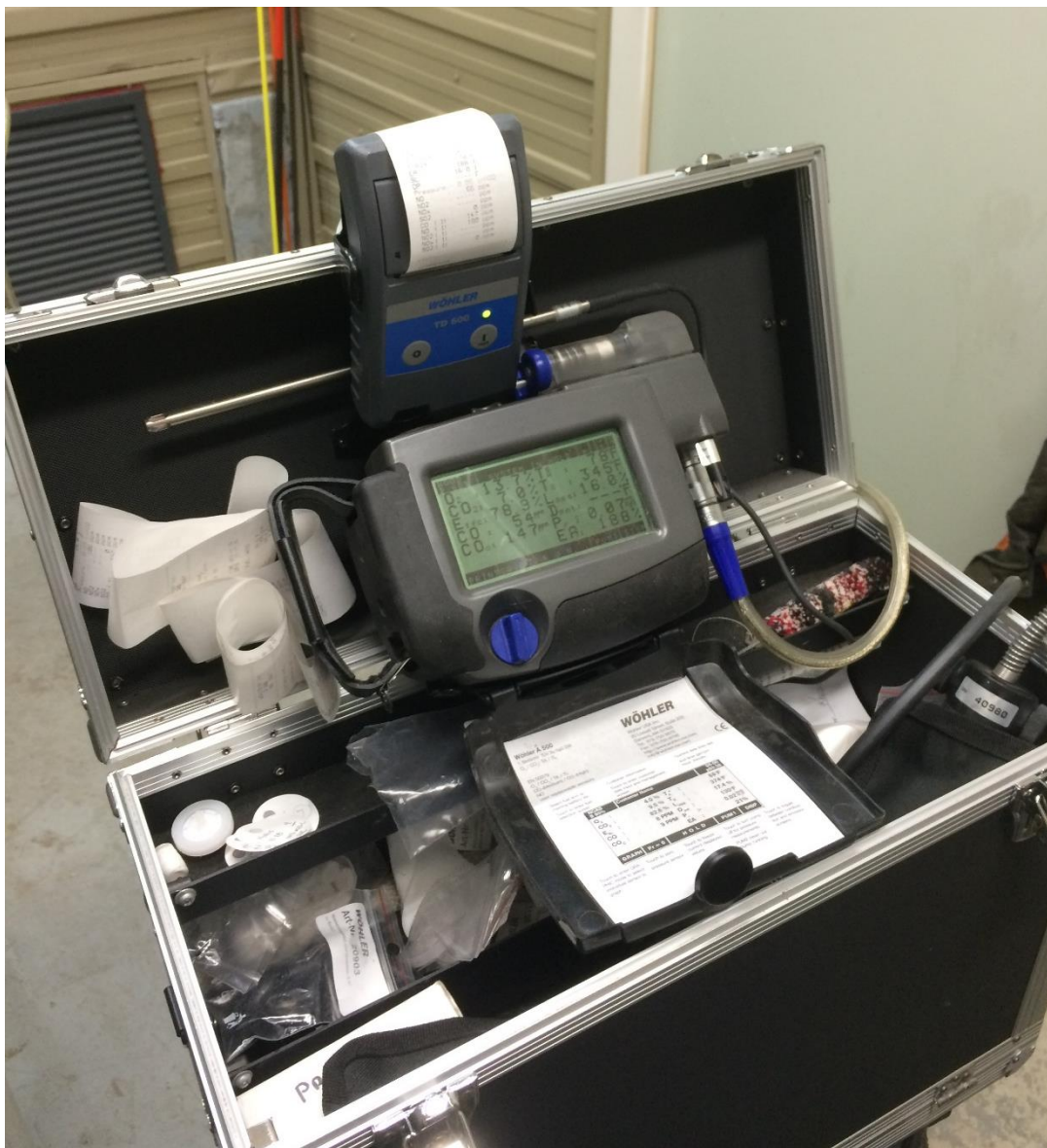
Figure 8 - A Wohler A500 combustion analyzer was used to measure the content and conditions of the combustion exhaust.
