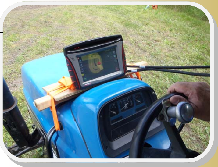
FM-750 GPS display for precision agriculture steering guidance.
