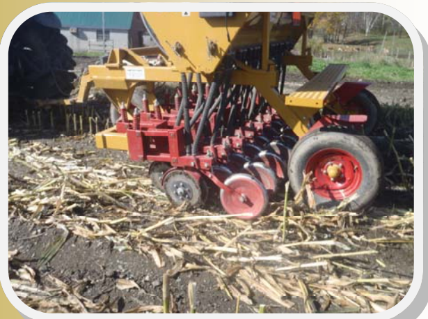
No-Tilling winter cover crops into corn ground after harvest is accomplished in one pass, saving energy by
