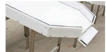
Spring-loaded lid in open position
