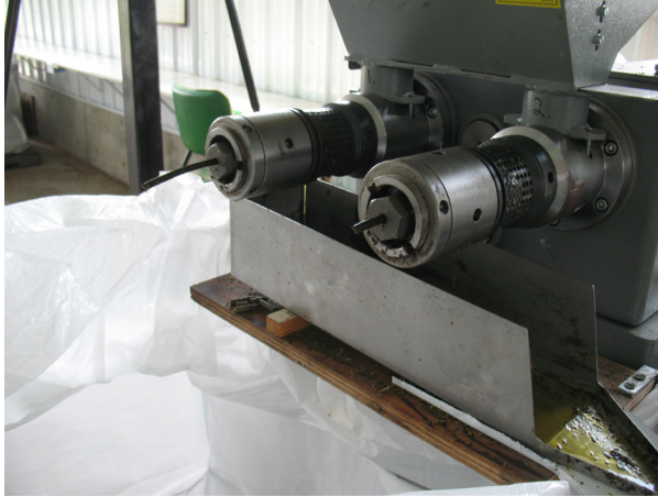
Borderview eventually abandoned the attended press for two automated presses used both for fuel production and for research trials.
