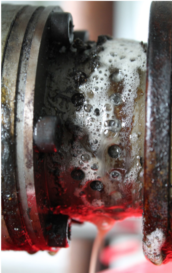
Oil presses are used to crush the seed and separate oil from the meal. In this picture the oil is seen coming through the wall of the press barrel, seed is coming in from the right via a screw impeller and meal leaves to the left.
