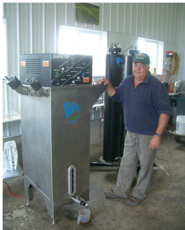
Roger Rainville (Alburgh) purchased a BioPro 190 biodiesel processor after careful consideration of building his own system. He liked the fact that the machine came all in one piece, "ready to go." Roger also bought a fuel finishing unit (background) that attaches to the BioPro to filter fuel and remove water and glycerin.
