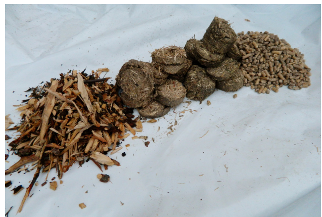
A variety of biomass fuels. Left to right: wood chips, grass pucks or briquettes, and wood pellets.
