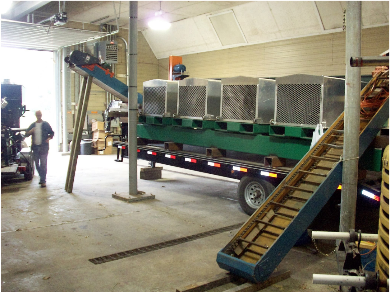
Renewable Energy Resources' Compactor 5000 is housed on a 25 ft trailer and is designed to be pulled by a 5-wheel with an optional \frac{3}{4} ton pick-up truck hookup. Enabling mobility makes the compactor an ideal option for growers and fuel suppliers who have multiple field locations.
