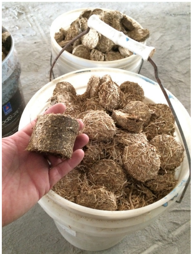
Fuel “pucks” made from Switchgrass by RER for combustion testing.
