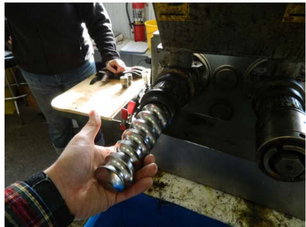
Changing screw impellers on the Kern Kraft press at Borderview Farm (Alburgh). Different screws are used for different seeds based on size and hardness.
