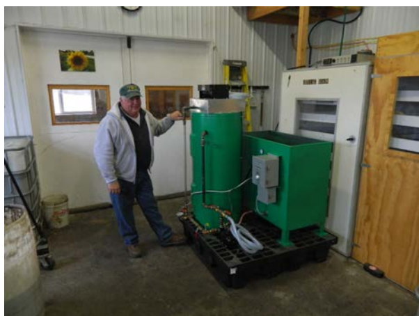
Roger Rainville shows off his methanol recovery system. Removing residual alcohol from the final fuel batch is an important quality hurdle that VBI funding helped to address.
