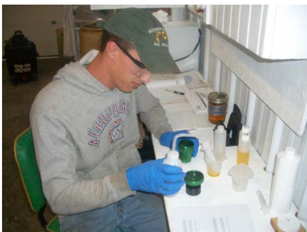
Jerrod LaValley performs a test for water in feedstock oil at Borderview Farm prior to making a batch of fuel. The VBI supported the purchase of simple lab equipment like this to improve fuel quality at the partner farms.
