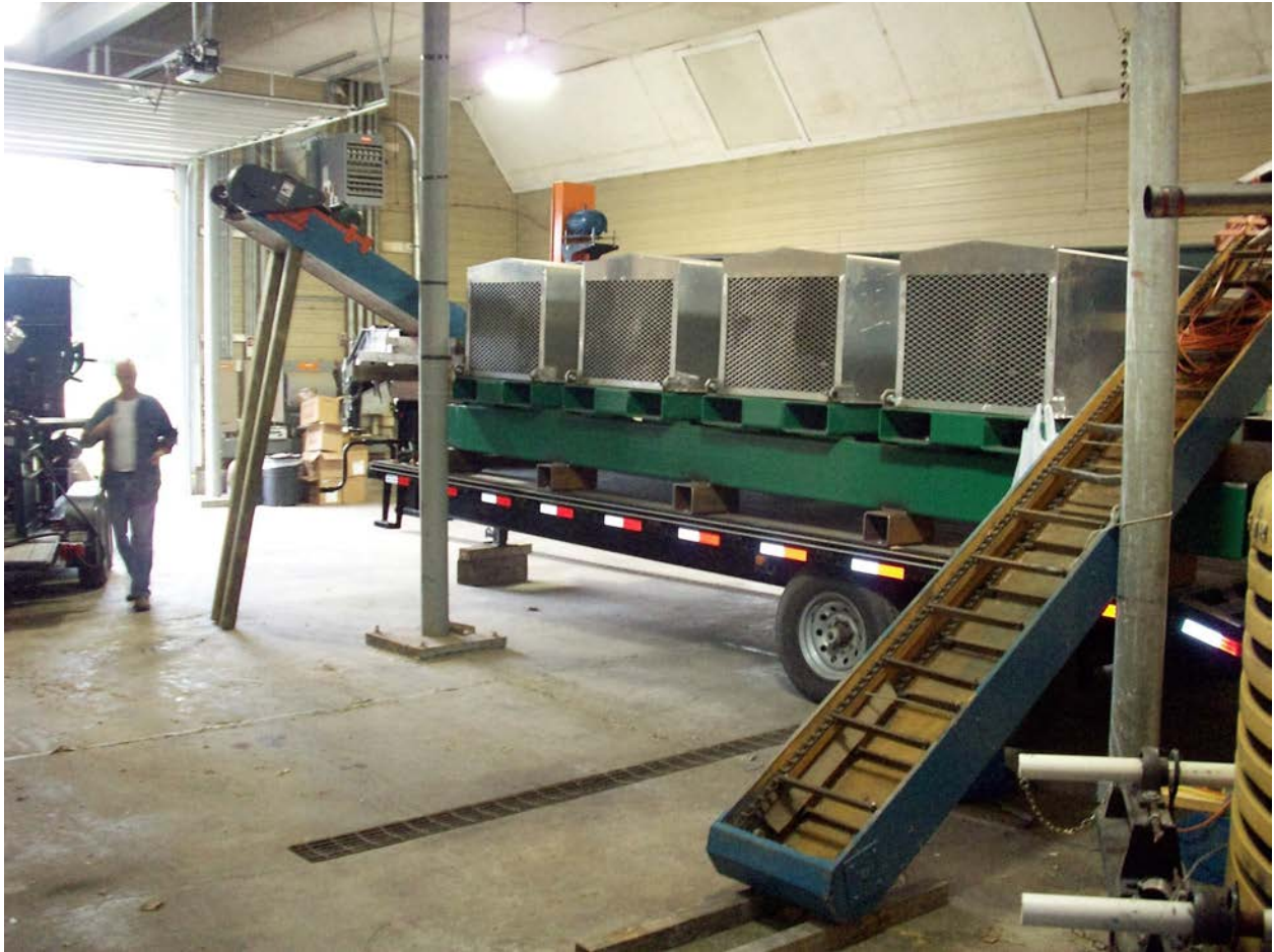
Renewable Energy Resources' Compactor 5000 is housed on a 25 ft trailer and is designed to be pulled by a 5-wheel with an optional ¾ ton pick-up truck hookup. Enabling mobility makes the compactor an ideal option for growers and fuel suppliers who have multiple field locations.
