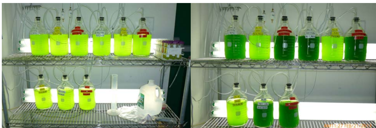
Flue gas experiment shows the visual impact of differences in cell density between air plus CO 2 (white labels), air only (yellow labels), and air plus flue gas (red labels) at time of stocking (left) and 48 hours later (right).
