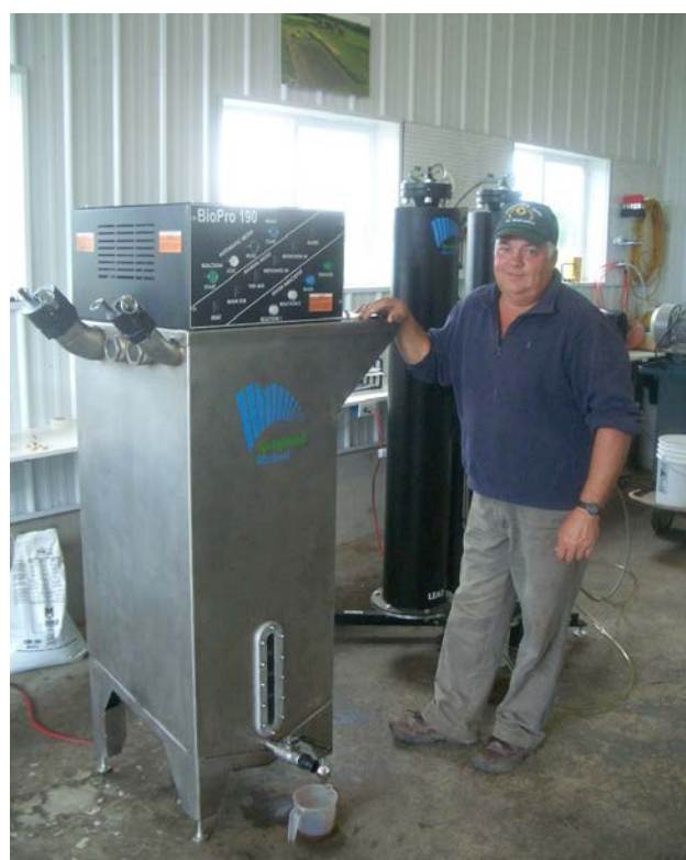
Roger Rainville (Alburgh) purchased a BioPro 190 biodiesel processor after careful consideration of building his own system. He liked the fact that the machine came all in one piece, "ready to go." Roger also bought a fuel finishing unit (background) that attaches to the BioPro to filter fuel and remove water and glycerin.
