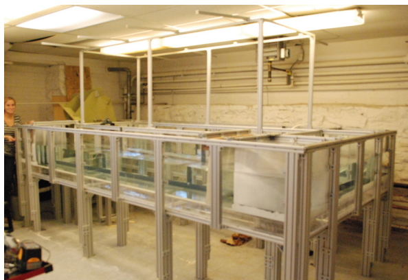
Overview of the flume filled with water. The lighting system suspended above the flume is not shown in this photo.
