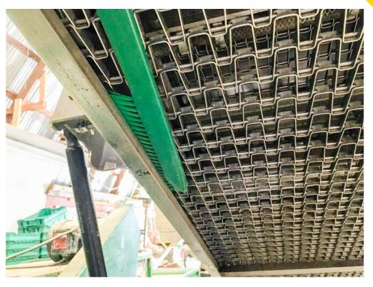
A narrow brush flosses the crack between the frame and the chain conveyor
