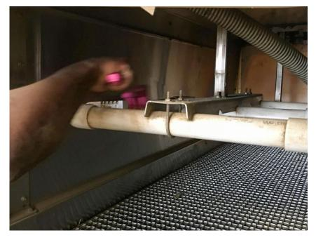
A long handed brush can make scrubbing the PVC assembly easier.
