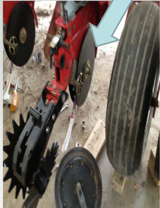
Installed heavy duty 3.5mm disk openers
